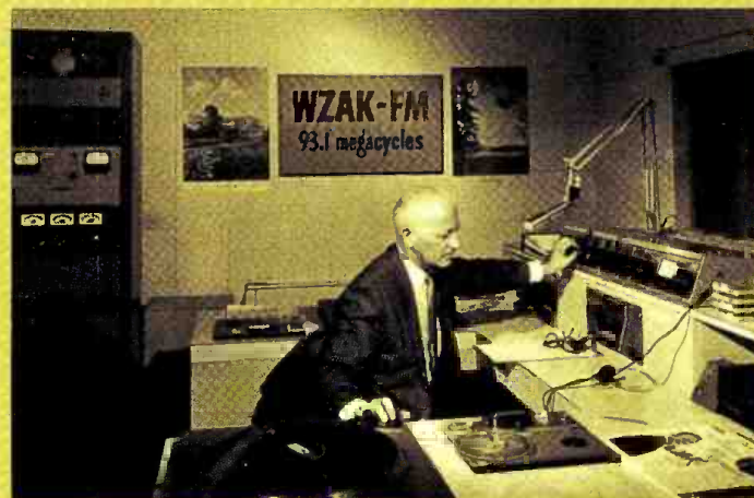
In radio broadcasting . . . stereo station WZAK-FM, Cleveland, Ohio, is fully equipped by Gates Radio division. Operating the Yard 8-channel speech input system is WZAK's general manager, Joseph Bauer. Control room is also equipped with two Gates turntables and tape-cartridge playbacks, a Gates recording amplifier, remote-control unit and FM transmitter.
